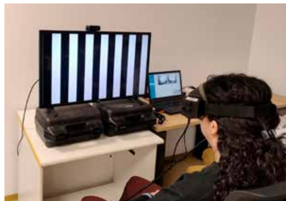
Figure 1. Experimental setup for videonystagmographic recording of eye movements. Participants were seated facing the recording screen while wearing VNG goggles (here, facing a moving visual pattern for optokinetic nystagmus examination).
